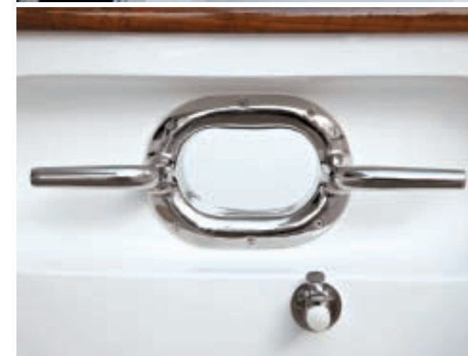
Top: Stairs leading from the pilothouse to the dinghy deck are nice and wide. The stainless handrail adds a feeling of security. Above: Hawse cleats are set into the side decks, which helps prevent stubbed toes.
